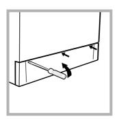
1. using a screwdriver, remove the cover panel on the lower front of the washing machine (see figure);
